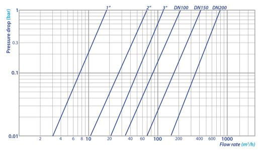
Head losses are referred to filters with 120  $\mu m$  clean filtering mesh.
